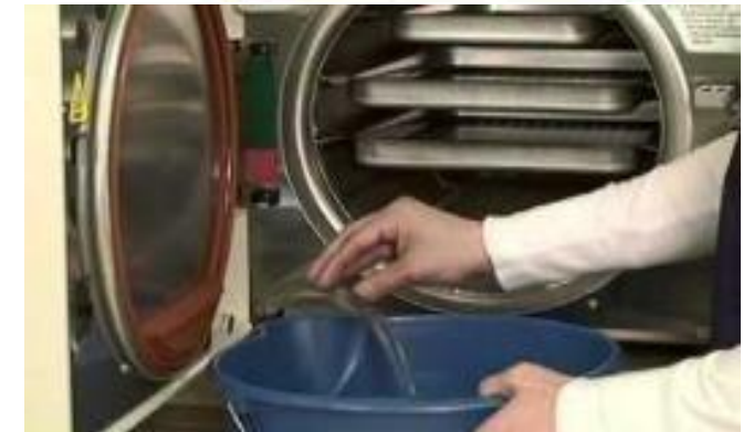
Steam Sterilizer – Draining Water
